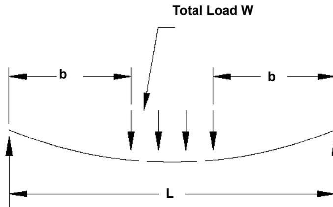
Figure 9 Beam Loading Conditions for Deflection Analysis
