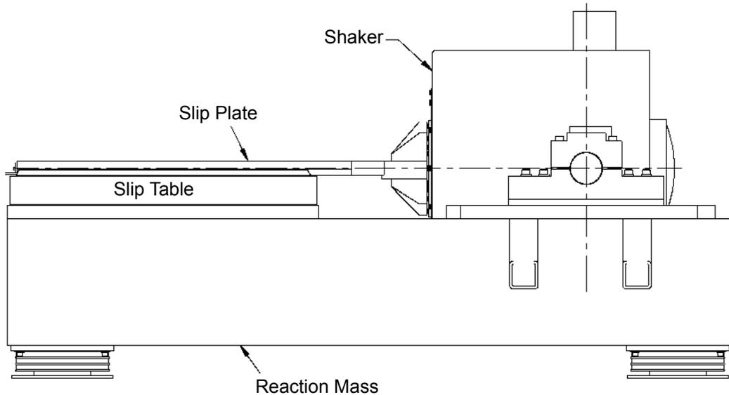
Figure 1 Typical Shaker and Slip Table System
