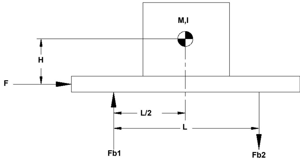
Figure 3b Free Body Diagram of Forces Acting on Slip Plate
