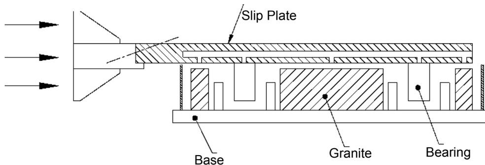
Figure 2 Cut-Away View of Journal Bearing Slip Table
