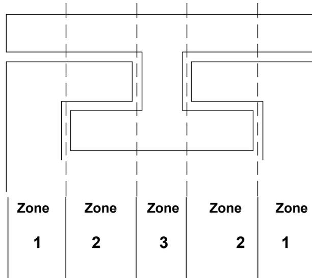
Figure 7a Stiffness Zones of T-Film Bearing Stiffness Model
