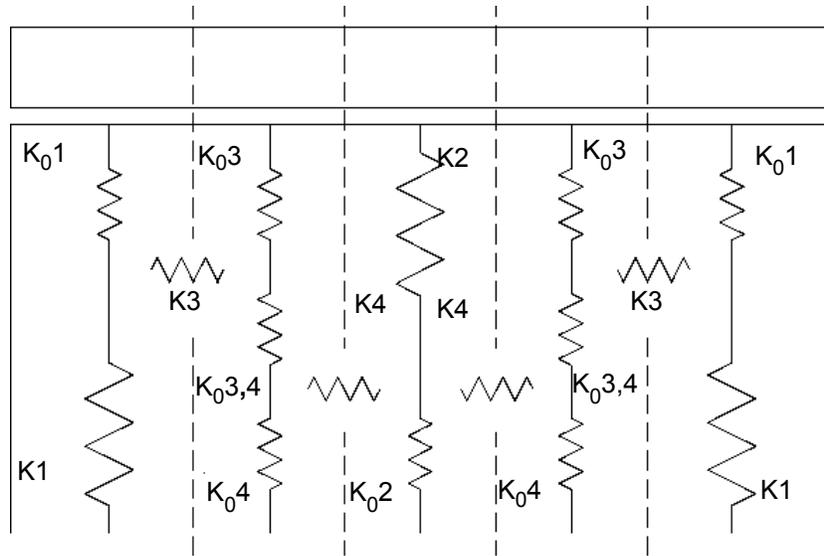
Figure 7b Spring Model of T-Film Bearing
