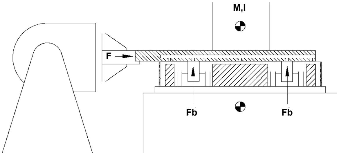
Figure 3a Forces Acting on Slip Plate
